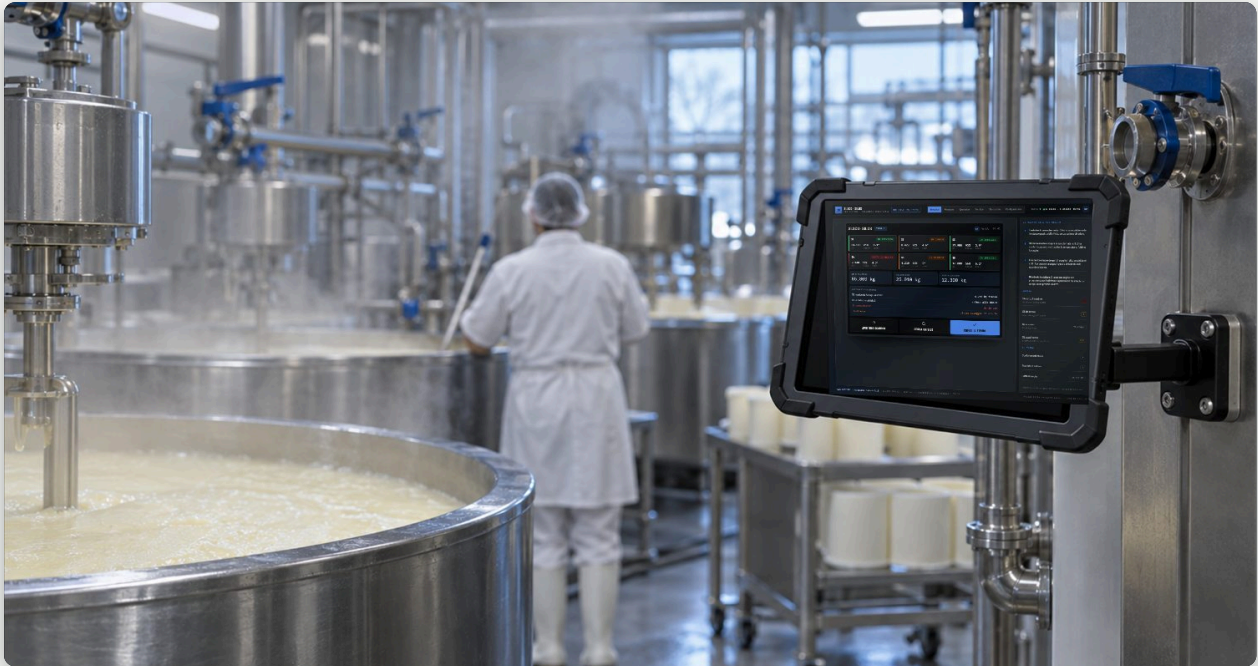
CHEESEMAKER TABLET The six silos on one screen, with weight, fill and temperature. Touching a silo opens its day; a discharge to the vat also opens from here.
